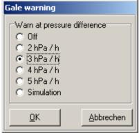
With fast changes of air pressure the gale danger is particularly high. In order to relieve you from the constant observation of the air pressure process, you can switch on the storm-warning. This function will be opened by the menu *Settings->Gale warning*.
